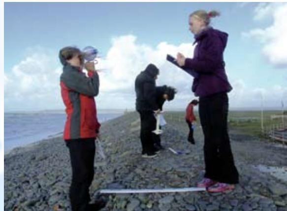
Pupils from Bideford College taking measurements of the pebble ridge. Sophie Bosworth is holding the clipboard. The girl facing her is holding a clinometer, a standard geography field device for measuring the angle of inclination of a slope. The girls in the background are holding calipers; these are used to measure the size and flatness of the pebbles both along the ridge and up and down the face.
