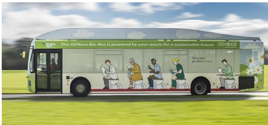
GENeco Bio-Bus, powered by biogas generated from sewage and food waste
