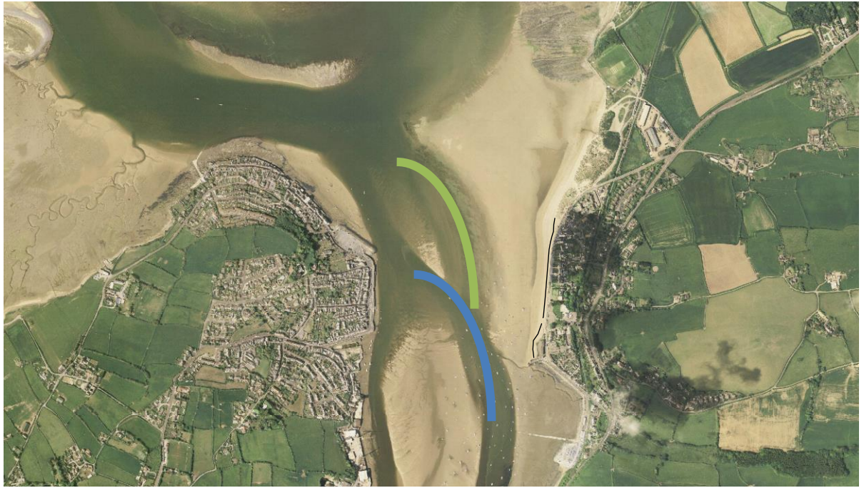
Figure: Primary Channel (blue) and secondary flood channel (green) locations in relation to beach. Maintaining a critical foreshore length will be important
