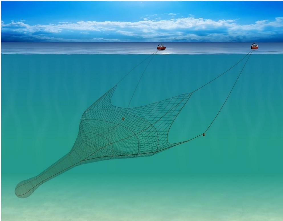
**Figure 17** - Pelagic pair trawl (Seafish, 2020c, <https://seafish.org/gear-database/gear/pelagic-pair-trawl/> [unedited]).
